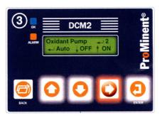
The default timeout for the forced ON condition is 10 minutes. After that delay, the relay will revert to AUTO mode. To adjust this time, refer to the install manual or ask your ProMinent Distributor for assistance.
