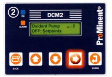
3. While holding the button, pressing one of the three other buttons , or will put the output in that respective mode.
