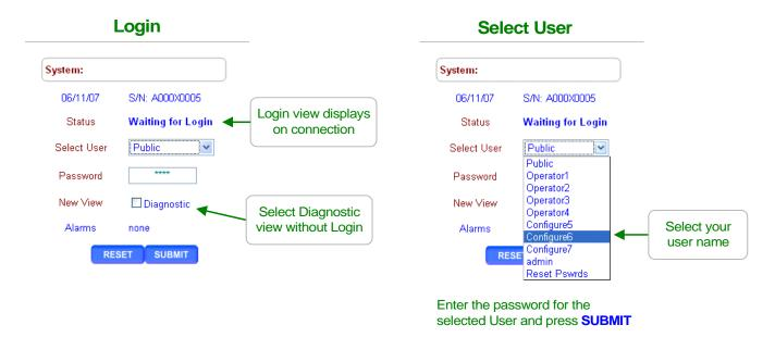
Once you've logged in, the controller's home page changes to show your user ID, **Current User**. Press the link at any sensor, meter, pump, solenoid or valve to view or modify.
