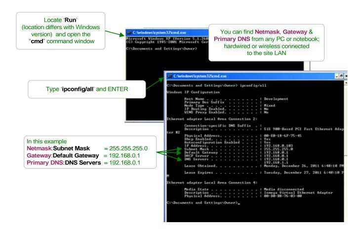
You can use either the Keypad-LCD interface or the browser to setup the controller's IP Address, Netmask, Gateway & Primary DNS.
