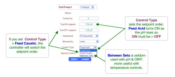
Each sensor pump control uses a **Control type** set by the chemical fed. ORP, pH and temperature sensors have **Control types** specific to the sensor.
