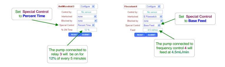
ON-OFF Pumps: Setting the % ON Time greater than 100%, sets the % to 100. 12% ON time is 36 seconds ON in every 5 minutes (0.12 x 300 seconds).
