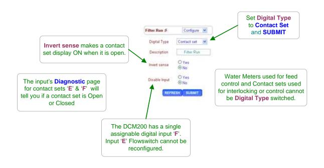
Sidebar: Volume & Contact Set Input: Controller input 'F' may be set to be a water meter or a contact set. The DCM200 is defaulted to contact at input 'F'.
